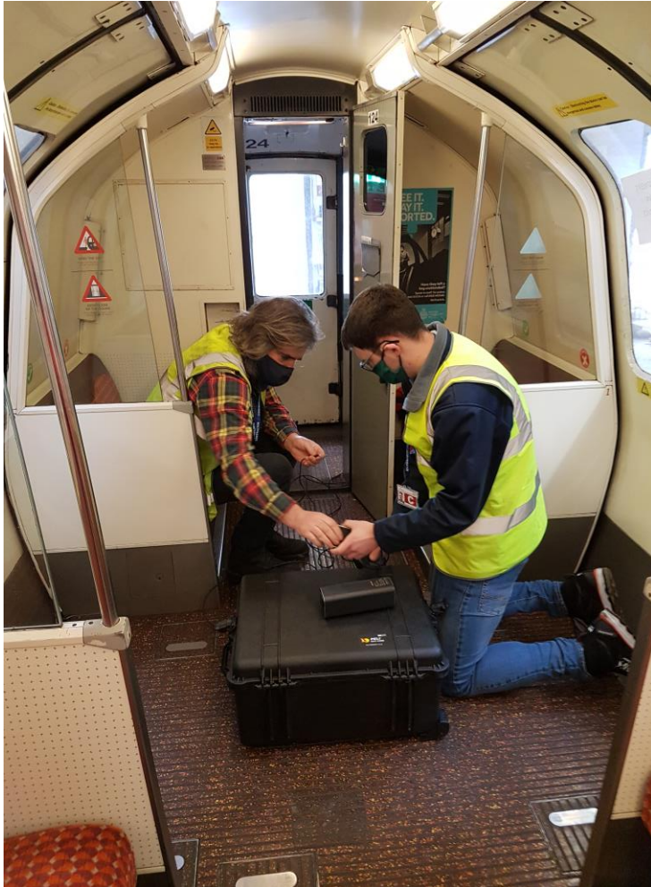
On-board network equipment placed in Peli Case
